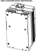
Step 3 Install a new fan in the VFD in the reverse steps. Assemble the VFD. Ensure the air direction of the fan is consistent with that of the VFD (blowing upwards).
