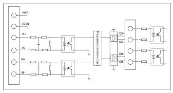
5. PG card frequency-divided open collector output connection
