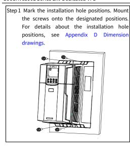
Step 2 Fix the VFD on the wall or mounting plate, and tighten the screws on the wall or mounting plate.
