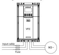
Figure 4-12 Fuse configuration
