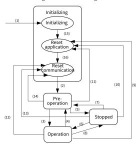
Figure 7-8 NMT state diagram
