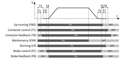
Figure 6-10 Timing sequence of maintenance running
