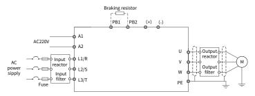
**Note:** The fuse, braking reactor, input reactor, input filter, output reactor, and output filter are optional parts. For details, see Appendix E Peripheral accessories.
