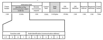
Figure 7-7 Packet structure
