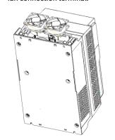
Step 3 Install a new fan in the VFD in the reverse steps. Assemble the VFD. Ensure the air direction of the fan is consistent with that of the VFD (blowing upwards).
