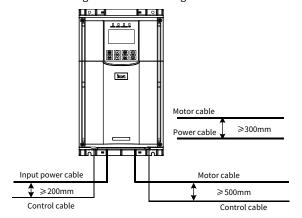
Figure 4-1 Cable routing distance
