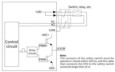
Figure G-1 Principle diagram of STO function
