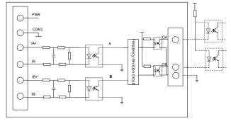
Note: During open collector output, PWR at J1 and that at J2 are short connected to COA and COB.
