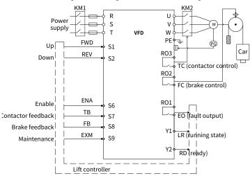
Figure 6-9 Wiring for maintenance running
