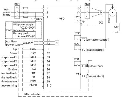
Figure 6-11 Wiring for emergency running
